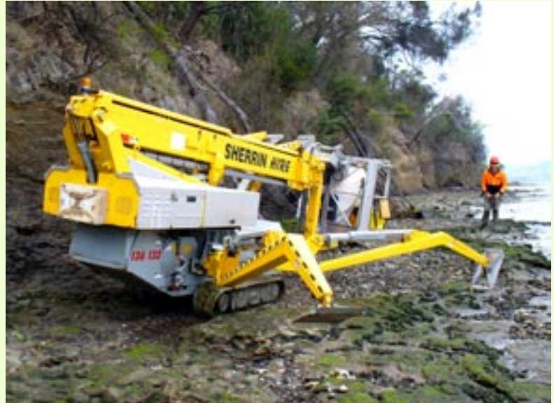
Glenn Szalman of Regnans enviro contracting "walking" the Spider via remote control (Photo by Di Harris)
